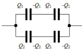
a) With the switch open, the charges on the capacitors distribute themselves as on Fig.3. The capacitance of the top line is the same as the capacitance of the bottom line (two capacitors in series)  $C_{top} = 2\mu\text{F}$ . From the symmetry we find that the charge will distribute itself evenly,  $Q_1 = Q_2 = Q/2$ . The total capacitance of the net of capacitors is  $C = 4\mu\text{F}$ . From
