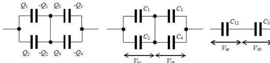
b) When we now close the switch, the situation will look like in the second picture. Because  $C_{12} = C_{34} = 9\mu\text{F}$  ( $C_{12}$  is  $3\mu\text{F}$  and  $6\mu\text{F}$  in parallel), we can easily see from symmetry, that  $V_{ac} = V_{cb}$ . So all the potential differences across all of the capacitors will be the same,  $V = V_{ac}$ ! How big are they?
