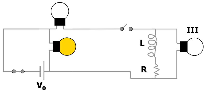
Energy stored in B-field is transformed into heat and light in R and bulb III
