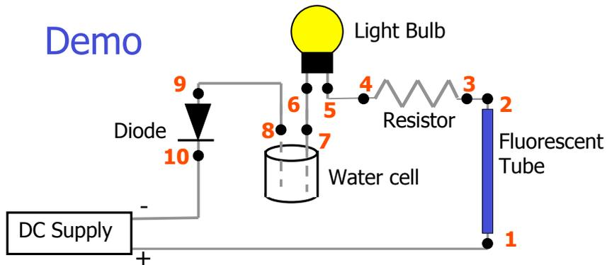
Output voltage  $V_{out} = V_{12} + V_{34} + V_{56} + V_{78} + V_{910}$
