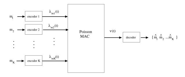
In extending Wyner's result from the single-user channel, Lapidoth and Shamai [4] showed that the capacity region for the Poisson MAC can be achieved by using input waveforms which are binary and which have infinitely-fast time variations. For the case of 2 encoders, Lapidoth and Shamai obtained the exact capacity region. In the general case of K users, they showed that the maximum total throughput is monotonically increasing in the number of users and that it is bounded from above.
