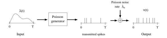
So there are two sources of noise in this channel: 1. the probabilistic nature in which spikes are generated at the transmitter, and 2. the extraneous spikes due to background emission (when referring to the generic Poisson channel, we will often use the term "spikes" instead of "photons"). More precisely, for an input  $\lambda(t)$ , the channel output in a small time increment  $(t, t + \Delta)$  has the distribution:
