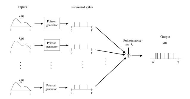
The output can simply be thought of as the superposition of the outputs of K independent single-user Poisson channels. That is, for inputs  $\lambda_1(t), \lambda_2(t), \ldots, \lambda_K(t)$  (where the
