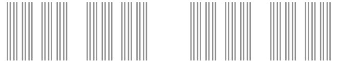
Fig. 6. The data bits are used to sequentially refine a point on a Cantor set. Its natural tree structure allows bits to be encoded sequentially. The Cantor set also has finite gaps between all points corresponding to bit sequences that first differ in a particular bit position. These gaps allow the uniformly reliable extraction of bit values from noisy observations.
