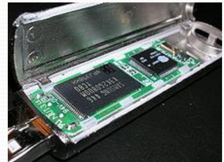
A USB Flash Drive. The chip on the left is the flash memory. The controller is on the right (Wikipedia).
