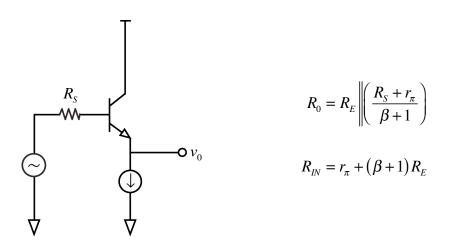
The output impedance depends on the source resistance. Unfortunate! Nevertheless, we can still incorporate this into our model framework. A stage is now:
