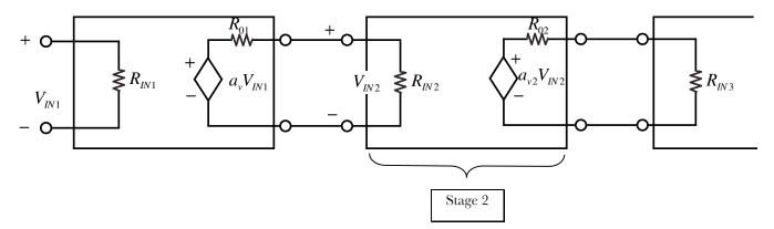
If stage 2 is an emitter follower,  $R_{IN2}$  is a function of  $R_{IN3}$ , and  $R_{O2}$  is a function of  $R_{O1}$ . Algebraically:
