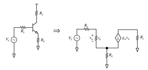
What we would like to do is somehow transform the network above to one that looks like the simple common-emitter stage. What does that mean, exactly?
