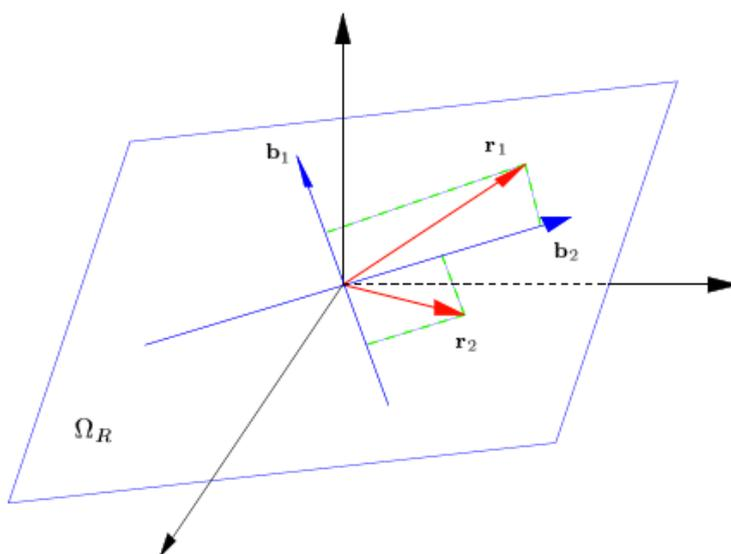
In high SNR regime, the effect of noise in the received signal is very small and we can study the signal  $\underline{Y}_0 = \underline{H} \underline{X}$  instead of  $\underline{Y}$ .
