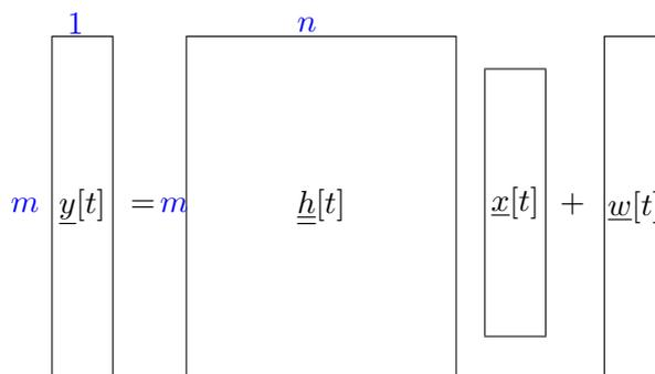
In *flat fading* MIMO communications, the matrix  $\underline{h}[t]$  is constant over a block of communication i.e.,  $\underline{h}[t] = \underline{H}$  for  $t = 1, 2, \dots, T$ .
