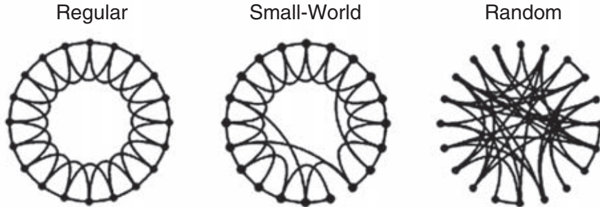
Figure 1: Diagram showing the relation among small-world network, regular network, and random network[1].
