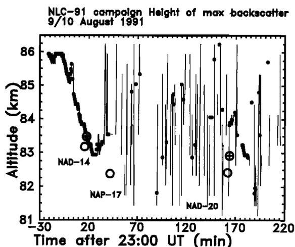
Fig 4. Comparison of the altitude of the maximum PMSE (radar) and NLC (in situ) signal strengths as a function of time. The heights of all the echoes were connected by a fine line. Whenever a sequence of four echoes was within  $\pm 500 \text{ m}$  around the average value at that time it is marked with a  $\bullet$ . The NLC data are given as  $\circ$  for the upleg and as  $\oplus$  for the downleg.
