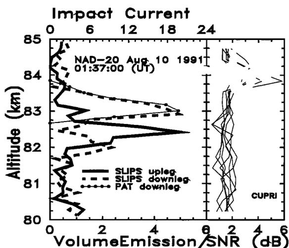
Fig 3. Data from the NAD-20 payload launched at 01:37:00 UT on August 10, 1991 (left). The SLIPS photometer and the PAT sensor indicate the height of the NLC layer. The units are arbitrary. Also shown are profiles of post-processing signal-to-noise ratio recorded by CUPRI (right). Note that the successive profiles from 01:44:09 to 01:48:05 UT with an integration time of 34 s. There was no PMSE layer in the radar volume at 01:37 UT.
