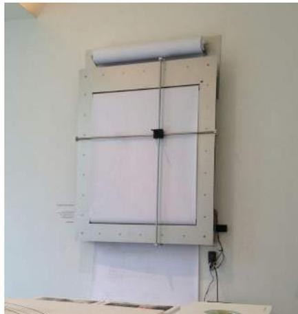
Figure 6. Wall-mounted Plotter (Source: Photography by Kim Sung Su)
