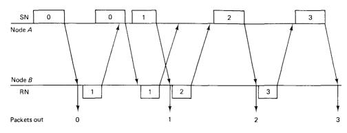
Figure 2.21 Example of use of sequence and request numbers for stop-and-wait transmission from A to B. Note that packet 0 gets repeated, presumably because node A times-out too soon. Note also that node A delays repeating packet 1 on the second request for it. This has no effect on the correctness of the protocol, but avoids unnecessary retransmissions.
