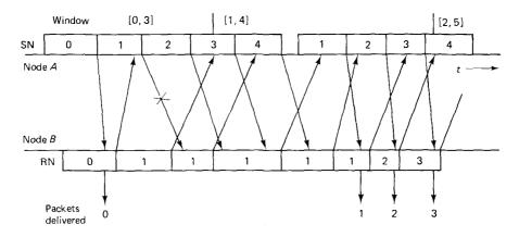
Figure 2.25 Effect of a transmission error on go back 4. Packet 1 is received in error at B, and node B continues to request packet 1 in each reverse frame until node Atransmits its entire window, times-out, and goes back to packet 1.
