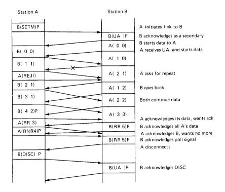
Figure 2.41 Asynchronous balanced mode (ABM) of operation. SETM refers to the set ABM command, which initiates the link with SN and RN at both sides equal to 0. Note the use of addresses in different types of frames.
