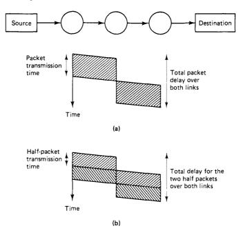
**Figure 2.37** Decreasing delay by shortening packets to take advantage of pipelining. (a) The total packet delay over two empty links equals twice the packet transmission time on a link plus the overall propagation delay. (b) When each packet is split in two, a pipelining effect occurs. The total delay for the two half packets equals 1.5 times the original packet transmission time on a link plus the overall propagation delay.
