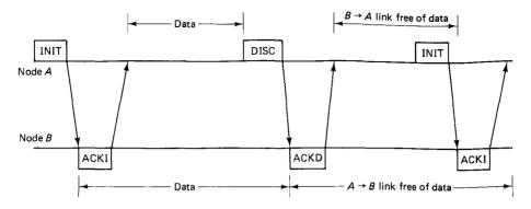
Figure 2.43 Illustration of periods when link is free of data in each direction. Note that the link is free in both directions both when A sends INIT and when B receives it.
