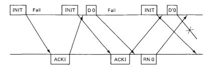
**Figure 2.46** Example of a sequence of node failures, with loss of state, that causes a failure in correct initialization. Each time the node recovers from a failure, it assumes that ACKD was the last protocol message received, thus allowing acknowledgments from earlier initialization periods to get confused with later periods.
