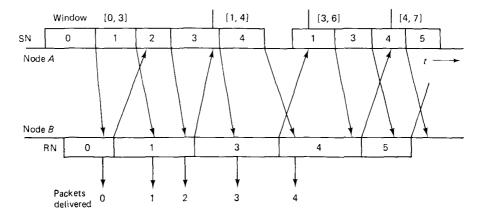
**Figure 2.27** Effect of delayed feedback for go back 4. The frames in the B-to-A direction are much longer than those in the A-to-B direction, thus delaying the request numbers from getting back to A. The request for packet 1 arrives in time to allow packet 4 to be sent, but after sending packet 4, node A times-out and goes back to packet 1.
