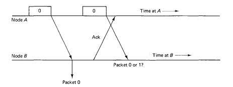
Figure 2.18 The trouble with unnumbered packets. If the transmitter at A times-out and sends packet 0 twice, the receiver at B cannot tell whether the second frame is a retransmission of packet 0 or the first transmission of packet 1.
