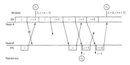
**Figure 2.28**  $SN_{min}$  is *i* at time  $t_1$ . Packet *i* is then released to the higher layer at *B* at time  $t_2$  and the window is increased at *A* at time  $t_3$ .
