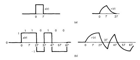
**Figure 2.3** Relation of input and output waveforms for a communication channel with filtering. Part (a) shows the response r(t) to an input s(t) consisting of a rectangular pulse, and part (b) shows the response to a sequence of pulses. Part (b) also illustrates the NRZ code in which a sequence of binary inputs  $(1 \ 1 \ 0 \ 1 \ 0 \ 0)$  is mapped into rectangular pulses. The duration of each pulse is equal to the time between binary inputs.
