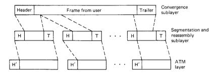
**Figure 2.57** Headers and trailers at the convergence sublayer and segmentation and reassembly sublayer of the adaptation layer. Note that the user frame and its convergence sublayer header and trailer need not completely fill the data area at the segmentation and reassembly sublayer. The data plus header and trailer at the segmentation and reassembly sublayer must be exactly 48 bytes in length, however, to fit into the ATM data area.
