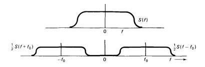
**Figure 2.10** Amplitude modulation. The frequency characteristic of the waveform s(t) is shifted up and down by  $f_0$  in frequency.
