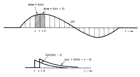
**Figure 2.5** Graphical interpretation of the convolution equation. Input s(t) is viewed as the superposition of narrow pulses of width  $\delta$ . Each such pulse yields an output  $\delta s(\tau)h(t-\tau)$ . The overall output is the sum of these pulse responses.
