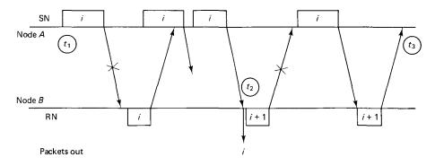
**Figure 2.22** Times  $t_1$ ,  $t_2$ , and  $t_3$  when a packet is first placed in a frame for transmission at A, first received and released to the higher layer at B, and first acknowledged at A.
