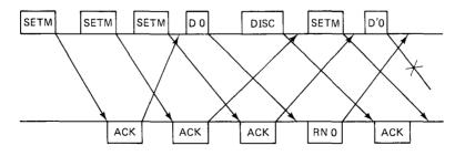
Figure 2.44 Example of HDLC in which node A attempts to initialize the link three times, due to delayed acknowledgments from B. The delayed acks are falsely interpreted as being acks for a subsequent disconnect and initialization. This in turn causes a failure in the data packets.
