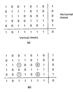
Figure 2.14 Horizontal and vertical parity checks. Each horizontal parity check checks its own row, and each column parity check checks its own column. Note, in part (b), that if each circled bit is changed, all parity checks are still satisfied.
