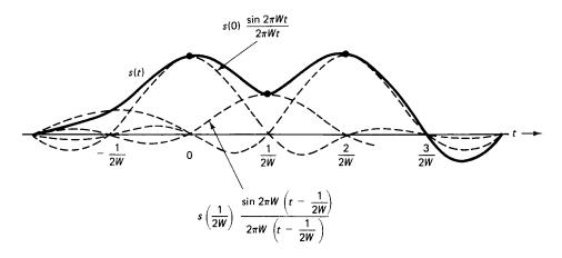
**Figure 2.6** Sampling theorem, showing a function s(t) that is low-pass limited to frequencies at most W. The function is represented as a superposition of  $(\sin x)/x$  functions. For each sample, there is one such function, centered at the sample and with a scale factor equal to the sample value.
