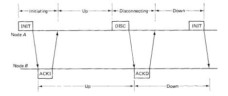
**Figure 2.42** Initialization and disconnection protocol. Data are transmitted only in up periods and the ARQ is initialized at the beginning of an up period. Note that node A cycles between periods of initiating, being up, disconnecting, and being down.
