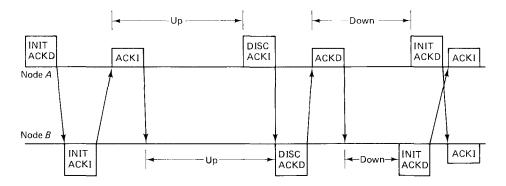
**Figure 2.45** Example of balanced initialization and disconnect protocol. Either node can start to initialize from the down state or start to disconnect from the up state and the other node will follow.
