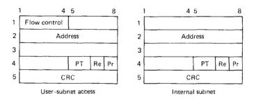
Figure 2.55 ATM header format for the user-subnet interface and for the internal subnet. PT stands for payload type, Re for reserved, and Pr for priority bit.
