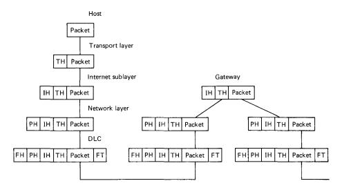
Figure 2.51 Illustration of a packet as it passes through a gateway. Within any given network, only the packet header and frame header are used, whereas at a gateway, the internet header is used to select the next network and to construct a new packet header appropriate to the new network.
