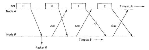
**Figure 2.19** The trouble with unnumbered acks. If the transmitter at A times-out and sends packet 0 twice, node B can use the sequence numbers to recognize that packet 0 is being repeated. It must send an ack for both copies, however, and (since acks can be lost) the transmitter cannot tell whether the second ack is for packet 0 or 1.
