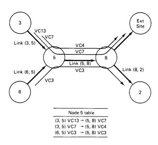
**Figure 2.47** Use of virtual channel (VC) numbers to establish virtual circuits in a network. Each packet carries its VC number on each link and the node changes that number (by a table representing the virtual circuit) for the next link on the path.
