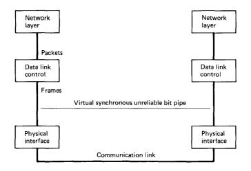
Figure 2.1 Data link control (DLC) layer with interfaces to adjacent layers.
