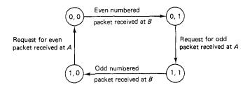
Figure 2.23 State transition diagram for stop-and-wait ARQ. The state is  $(SN \mod 2 \text{ at } A, RN \mod 2 \text{ at } B)$ .
