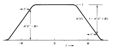
**Figure 2.7** Frequency response H'(f) that satisfies the Nyquist criterion for no intersymbol interference. Note that the response has odd symmetry around the point f = W.
