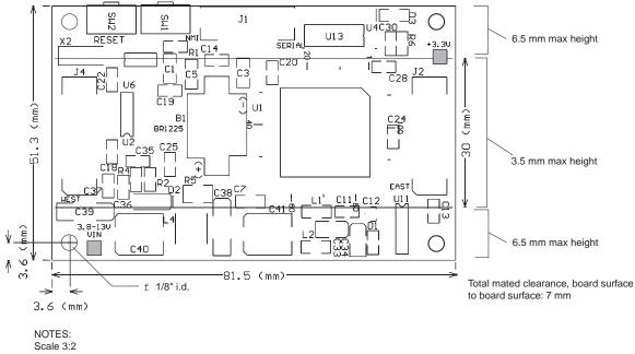
Scale 3:2 All dimensions within +/- 0.1 mm Important test points highlighted in gray
