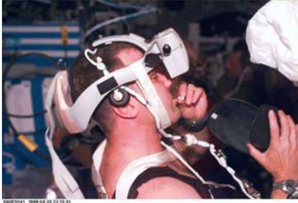
Figure 1. In-flight photograph of the HMD in operation aboard Neurolab. The communication headset worn underneath the HMD will be replaced with an integrated microphone and earphones. The shroud covering the HMD is in the crewmember's right hand.
