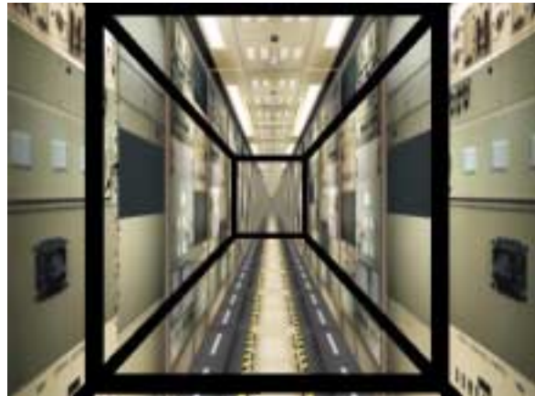
Figure 6. Neurolab version of the linear vection stimulus. Background scene moved toward subject. Black frame in foreground was stationary relative to the subject.
