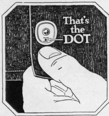
Lift dotted side of socket to release
