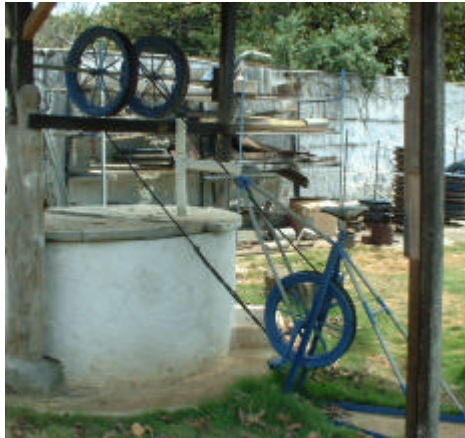
Figure 2. Rope pump well
