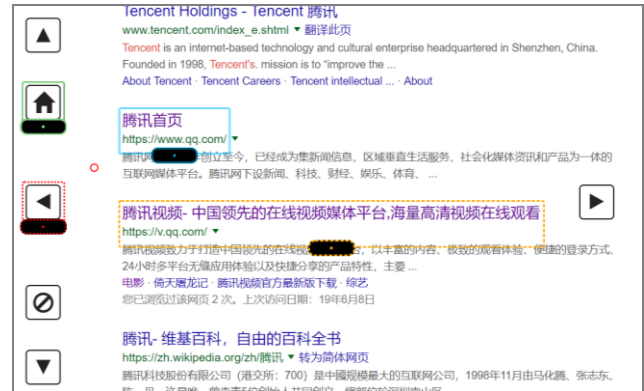
Fig. 1. GUI of our hybrid BCI web browser with 6 function buttons. The small red circle indicates the eye gaze point for clarity. Activated elements are bordered with a unique visual style.
