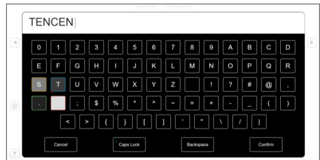
Fig. 2. Typing the last “T” of keyword “TENCENT” in the pop-up speller dialog. The buttons are flickering to provide the visual stimulation.
