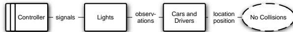
Figure 2. A problem diagram describing the domains and phenomena for a two-way traffic light. The arc connecting two domains is labeled by the phenomena shared by those domains – those phenomena that both domains involve. The arc connecting the requirement to a domain is labeled by the phenomenon referenced (constrained) by the requirement.
