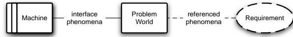
Figure 1. A generic problem frames description showing the disconnect between the phenomena controlled by the machine (the interface phenomena) and those constrained by the requirement (the referenced phenomena).
