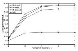
Fig. 10. Average capacities in a network with 20 nodes.
