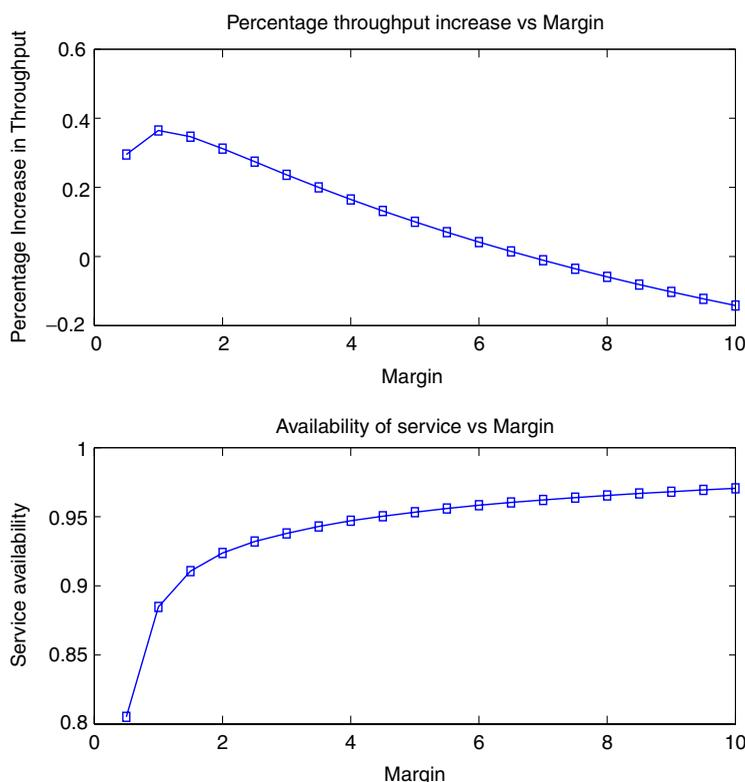
Figure 4. The percentage throughput increase (as compared to the CRT scheme) and availability in the adaptive rate transmission scheme with a constant margin.
