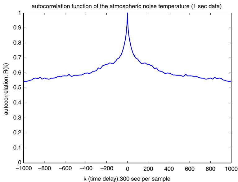
Figure 12. The autocorrelation function of the atmospheric noise temperature data with sampling interval of 5 min.
