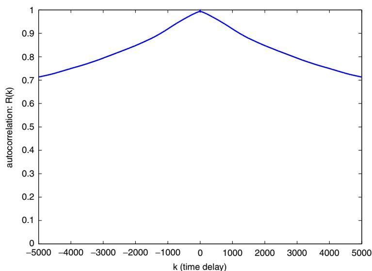
Figure 11. The autocorrelation function of the atmospheric noise temperature data with sampling interval of 1 s.
