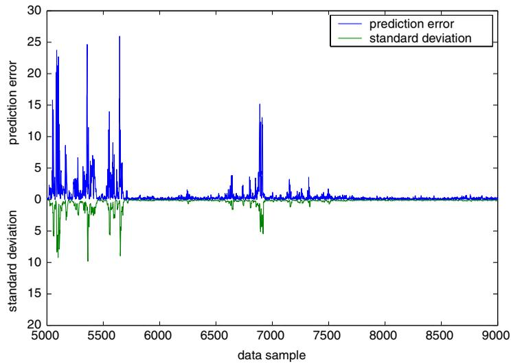
Figure 5. The correlation between the standard deviation of past measurements and the prediction error.
