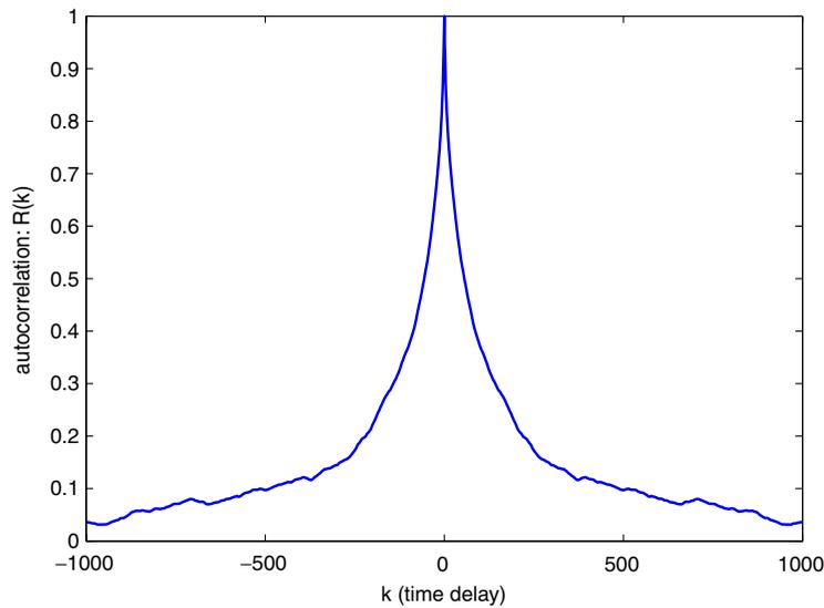
Figure 3. The autocorrelation function of the atmospheric noise temperature data with sampling interval of 5 min.
