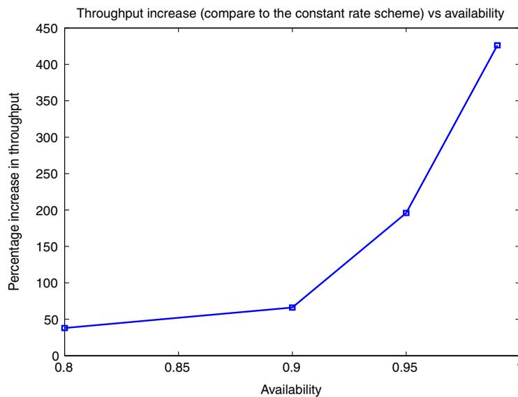
Figure 1. Percentage throughput increase of ART scheme over CRT scheme for different link availabilities.
