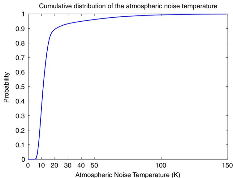
Figure 2. The cumulative distribution function of  $T_{\text{atm}}$ .
