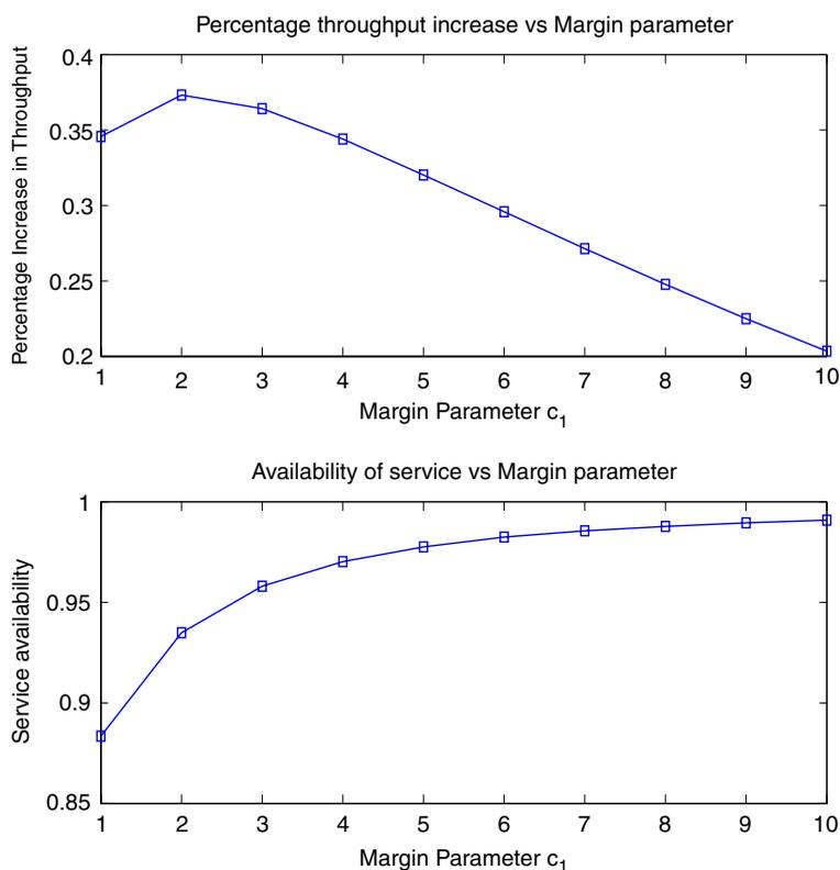
Figure 7. The percentage throughput increase and availability in the adaptive rate transmission scheme with an adaptive margin.
