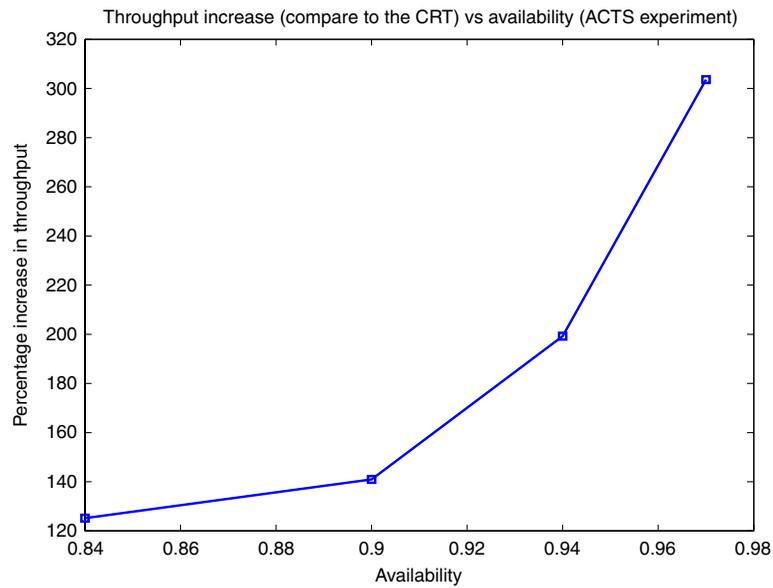
Figure 13. Percentage throughput increase of ART scheme over CRT scheme for different link availabilities.
