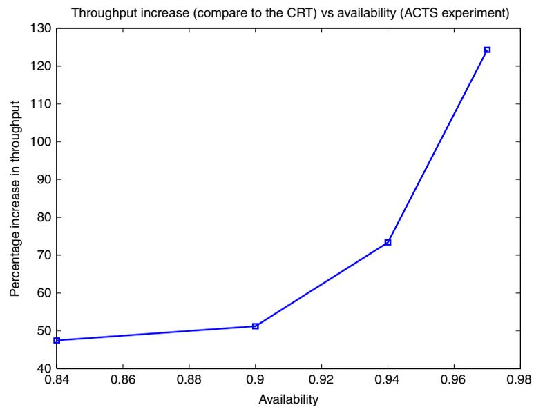
Figure 14. Percentage throughput increase of ART scheme over CRT scheme for different link availabilities with  $T_{eq} = 25$  K.
