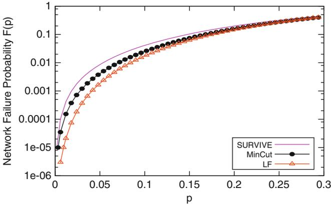
**Fig. 12.7** Network failure probabilities of three different lightpath routing algorithms
