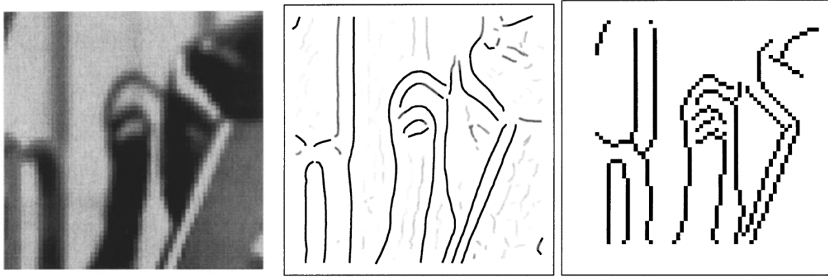
Fig. 1. Curve-based representations of image contours computed by the proposed approach (middle) and by more traditional methods (right). The edge representation on the right has been computed by using the Canny's algorithm implementation of the Matlab's image processing toolbox.
