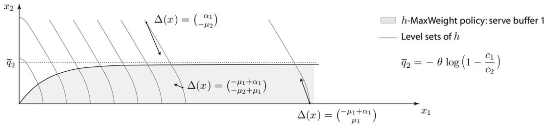
Figure 3: The perturbed cost function defined in (17) with  $h_0$  linear on  $\mathbb{R}^2$  satisfies  $\min_u \langle \nabla h(x), Bu + \alpha \rangle < 0$  for each non-zero  $x \in \mathbb{R}_+^2$ . This geometry is illustrated in this figure using the tandem queues. The contour plots shown are the level sets  $\{x : h(x) = r\}$  for  $r = 1, 2, \dots$
