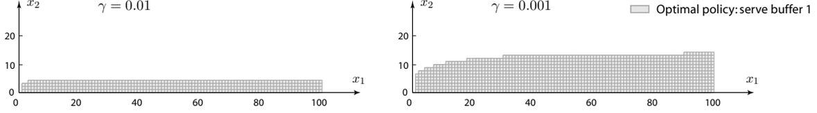
Figure 4: Discounted cost optimal policy for the tandem queues with cost parameters  $(c_1, c_2) = (1, 3)$ . The load parameters are  $\rho_1 = 9/10$ ,  $\rho_2 = 9/11$ , and the linear cost defined by  $c_1 = 1$ ,  $c_2 = 3$ . On the left  $\gamma = 0.01$  and on the right  $\gamma = 0.001$ .
