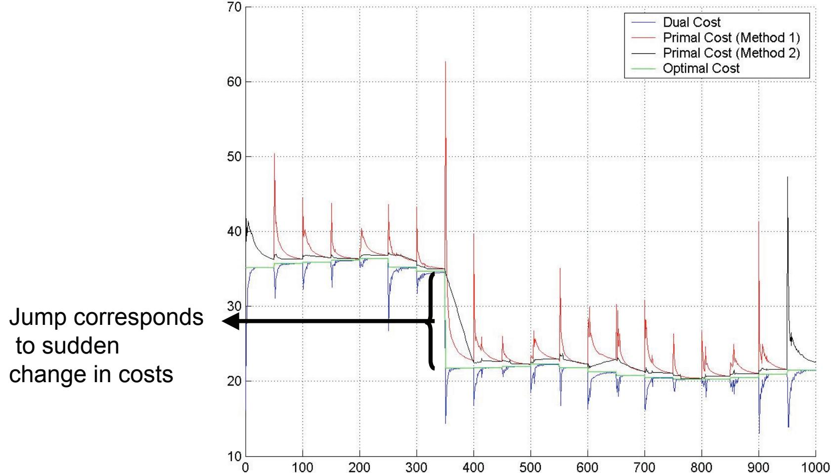
The black line tracks the optimal cost closely – the blue and red lines, although they correspond to techniques that also converge, do not provide the smooth behavior of method 2
