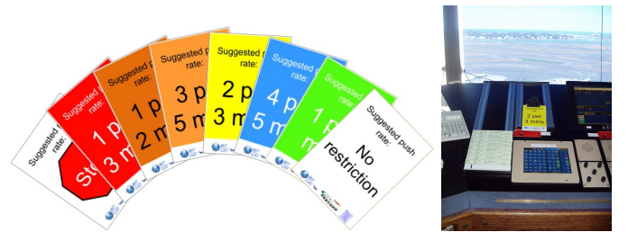
Fig. 7: (Left) Color-coded cards that were used to communicate the suggested pushback rates. (Right) Display of the color-coded card in the Boston Gate controller’s position.
