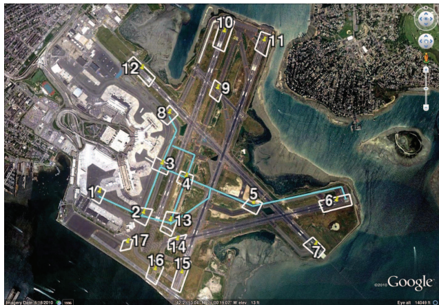
Fig. 1. Layout of the surface at BOS. Nodes in the network model are marked with white boxes. The configuration-specific network for departures from Runway 27 has been highlighted in blue.
