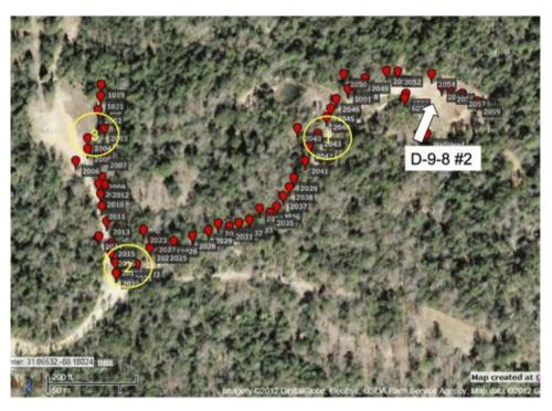
Figure 5 Location map of Citronelle MBM DAS testing. The MBM well, D-9-8 #2, is labelled with an arrow. Shot points for VSP are shown in red, with three DAS test focus points shown in yellow labels 1, 2, and 3. SP 2021 was the primary source location (yellow circled 2) with an offset of about 250 m (a near-zero offset for the geophones at about 2-km depth).
