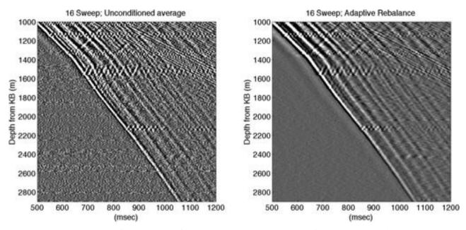
Figure 6 A randomly selected set of 16 DAS sweeps for SP 2021, comparing (left) stacking of native DAS data with (right) DAS data with adaptive stacking and spectral rebalancing.
