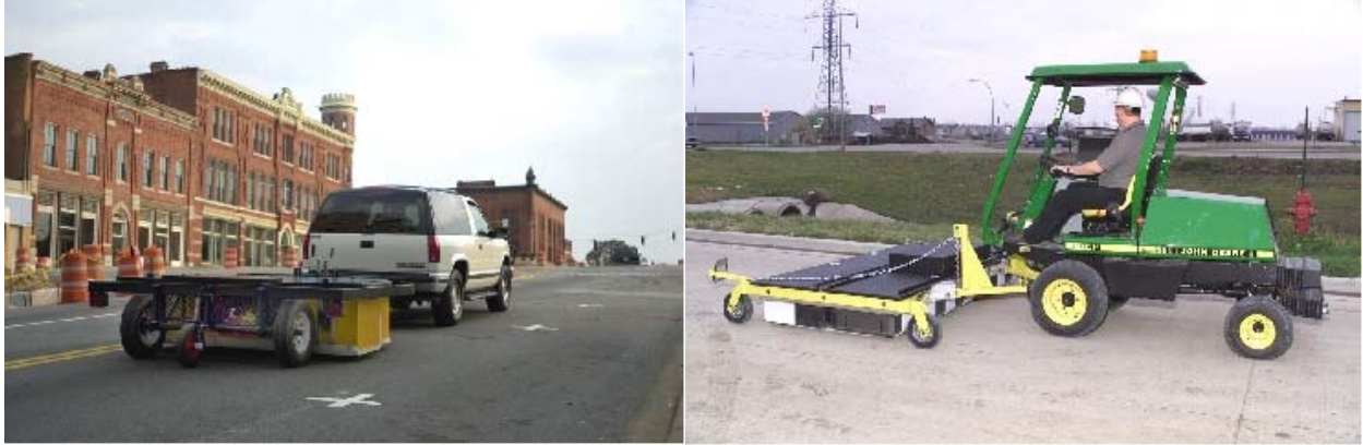
Figure 1: The radar array in the CART Imaging System can be deployed in a trailer that is towed by a vehicle (left) or in a special deck mounted in front of a commercial riding lawnmower (right).
