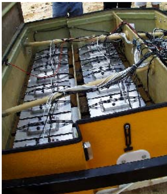
Figure 2: (Left) Photo inside the CART trailer housing the 17 radar antennas. (Right) Schematic top view of CART antenna array, which distributes 16 standard GPR channels over a 2 m swath considering a bi-static fixed offset data acquisition mode.
