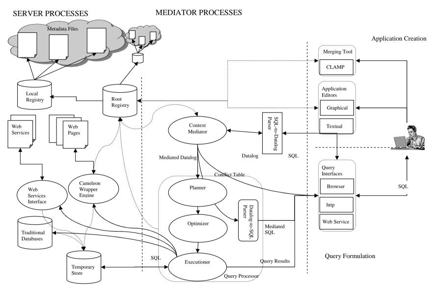
Figure 8.1 The ECOIN Prototype Architecture
